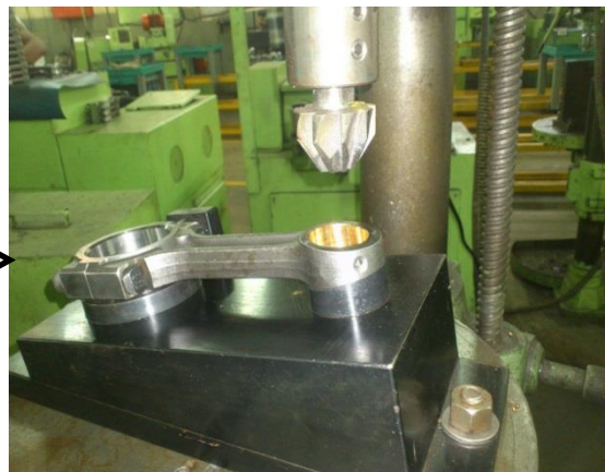
FIGURE 4.2 : Small End Bush Chamfering with Pillar Drill (After Implementation)
